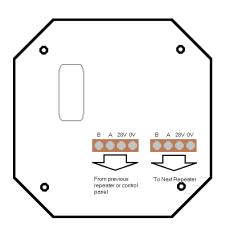
Two terminal blocks are provided on the back of the PCB to facilitate the installation of multiple repeaters. The panel can be connected to either of these terminal blocks.
