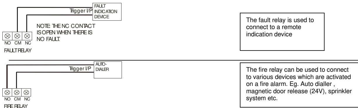
Typical auxiliary output wiring
