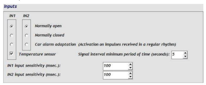
The module has 2 contact inputs: IN1 and IN2. The external contact is considered between the input and the negative terminal of the supply voltage input ("—" terminal).
