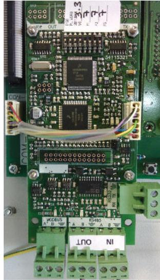
The Modbus Network Card has an RS485 repeater connection, an RS232 printer connection and a Modbus serial communications protocol connection.
