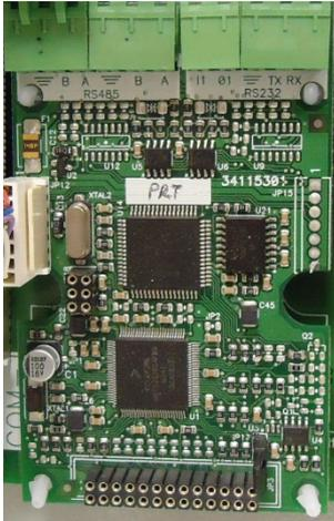
The Standard Network Card provides an RS485 repeater connection, and an RS232 Printer connection.
