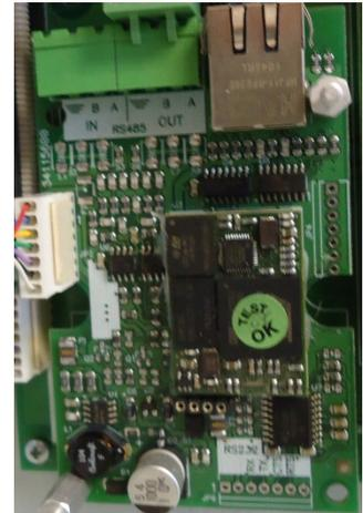
The Gateway Network Card has an RS485 repeater connection and a TCP/IP Interface for connection to the Data log Alarm Manager Software.
