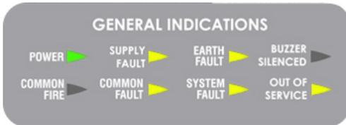
SUPPLY FAULT, COMMON FAULT, EARTH FAULT, SYSTEM FAULT, OUT OF SERVICE FAULT, which can be found at the top right of the LED display as shown.
