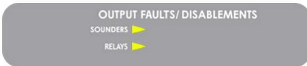
Two blocks below this in the section headed OUTPUT FAULTS / DISABLEMENTS are 2 LEDs which notify the user of SOUNDER FAULTS and RELAY FAULTS.
