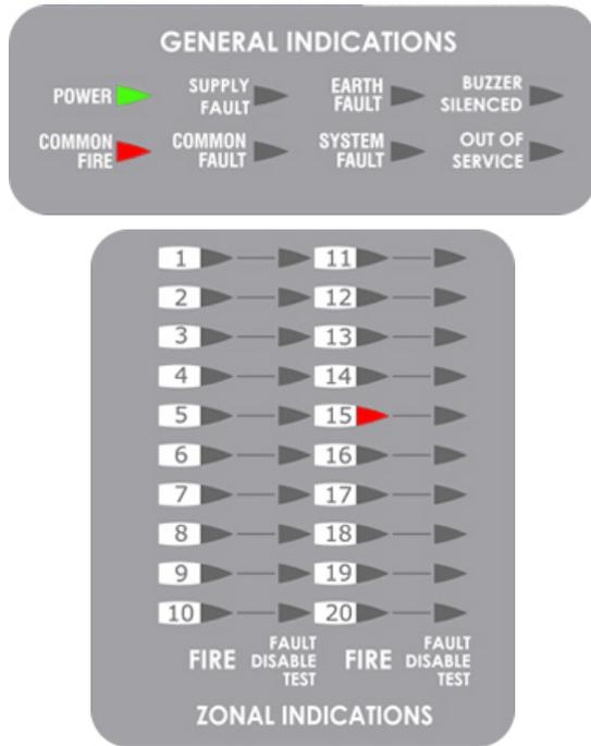
When the Panel is set into alarm by a Detector or Manual Call Point located in a zone that is not already in alarm it will: -
