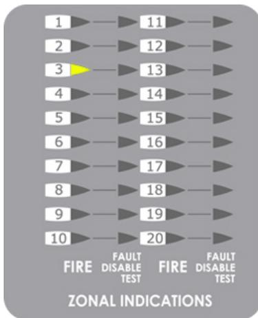
To the left of this are 20 LEDs which are used to indicate Zone Faults / Disablement / Test in Zones 1 – 20.
